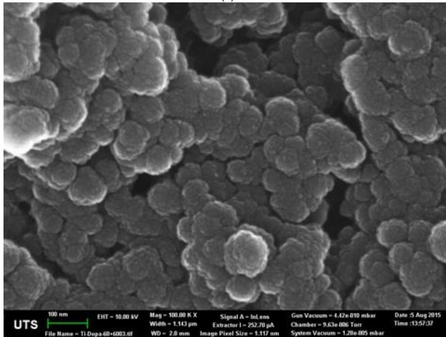
**Figure 3.** SEM micrographs showing (a) the Ti6Al4V surface with a polydopamine (pDA) coating (left) and uncoated (right) at a magnification of 1000 $\times$ , as well as (b) the pDA coating at 100,000 $\times$  magnification.
