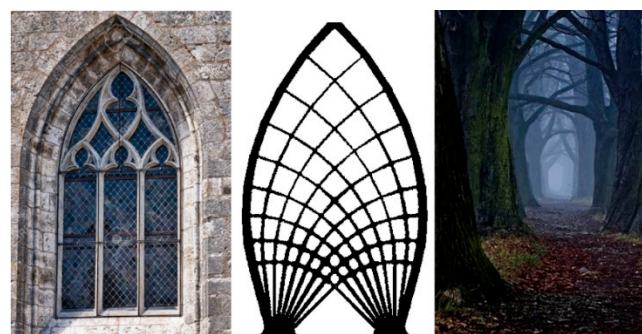
Figure 18. Gothic vaults in the shape of the Michell’s ideal truss contour and the nature-inspired interpretation.
