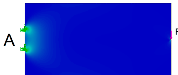
Figure 8. Load and joint of the base beam A (stress diagram).
