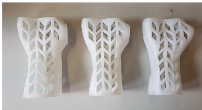
Figure 11. Orthoses manufactured vertically from nylon, strategies. (left to right) Econo, accura, strong.
