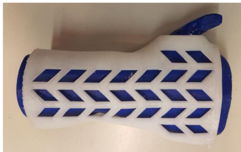
Figure 7. Orthosis on a two-material forearm phantom.
