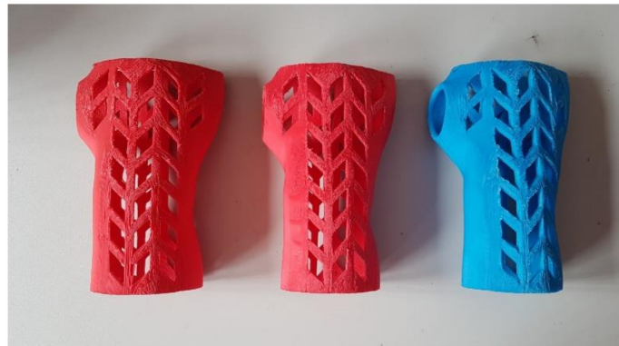
Figure 10. Orthoses manufactured horizontally from ABS, strategies. (left to right) Econo, accura, strong.
