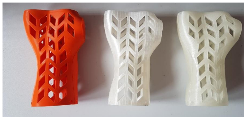
Figure 9. Orthoses manufactured vertically from PLA, strategies. (left to right) Econo, accura, strong.
