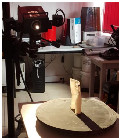
Figure 6. Measurement of an orthosis with a 3D scanner.
