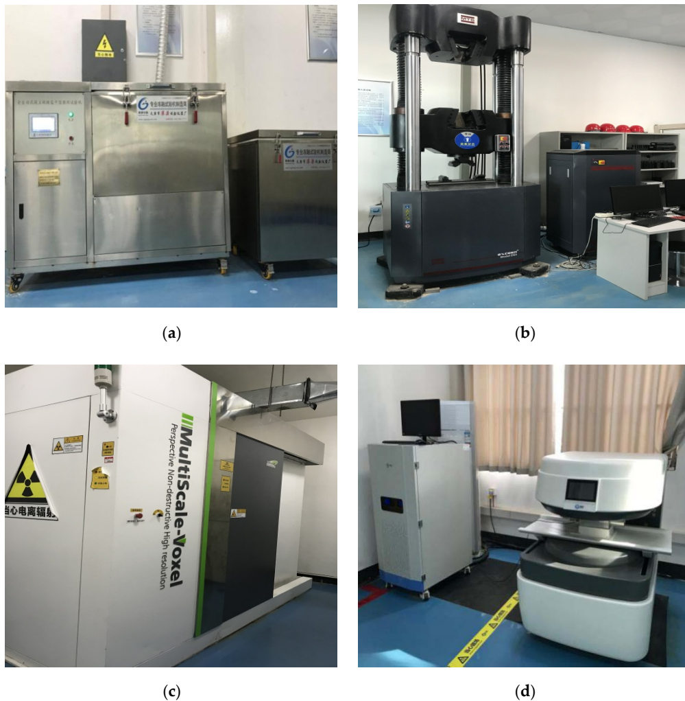
Figure 1. Test instruments and equipment: (a) The fully automatic machine for dry-wet circulation of sulfate; (b) MTS universal testing machine; (c) ICT; (d) The MacroMR 12-150H-I instrument.
