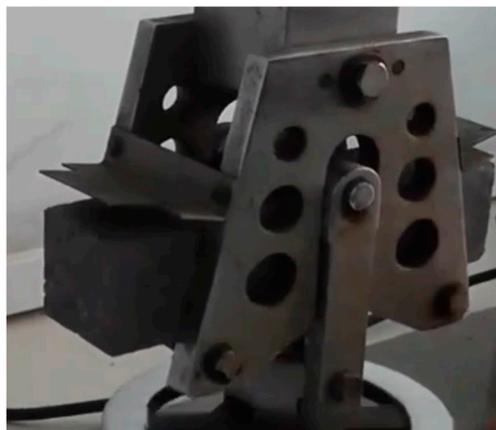
**Figure 2.** Specimen being fixed in the holder of the electric flexure tester.
