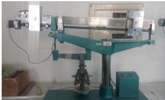
**Figure 1.** Electric flexure tester.
