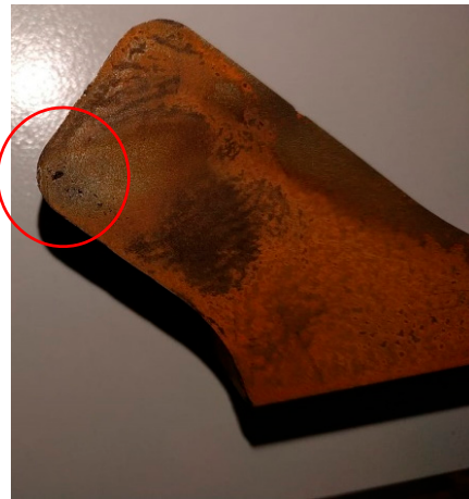
Figure 9. Defects located at the very end of the last filling regions (unfilled regions) of Trial 3.
