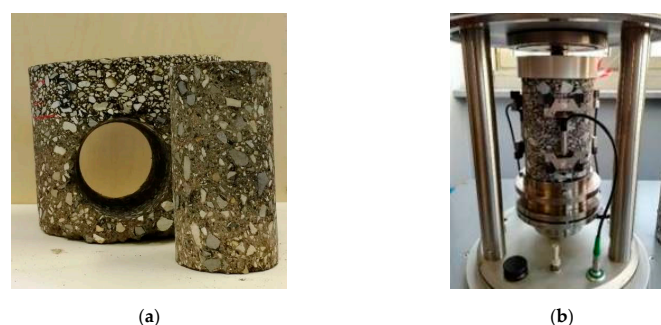
Figure 8. (a) Horizontal coring from core of 200-mm diameter; (b) detail of the specimen mounted in the asphalt mixtures performance tester (AMPT Pro).
