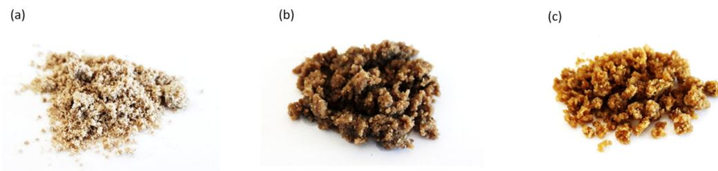
**Figure 1.** Hemp shives (HS) fillers used as reinforcing fillers: (a) non-treated hemp shives (HS), (b) hemp shives impregnated with sunflower oil (HS/SO), and (c) hemp shives impregnated with tung oil (HS/TO).
