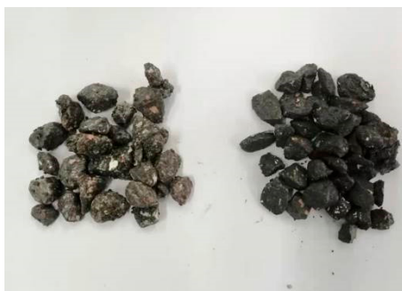
Figure 1. New iron-carbon-loaded substrate.
