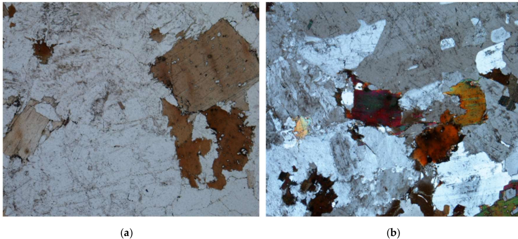
Figure 2. (a) Big biotite crystal with zircon inclusions and feldspar crystals (white light X64). (b) Quartz altered feldspars and biotite crystals (polarized light X64).
