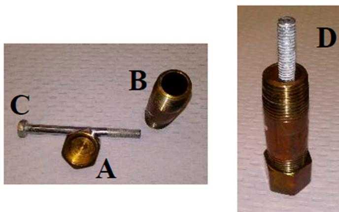
**Figure S3.** The bone crusher was made using three components. The bottom part (A) screws on to the barrel (B). The piston (C) then can be used to pulverize the bone using a hammer. (D) is the finished crusher.
