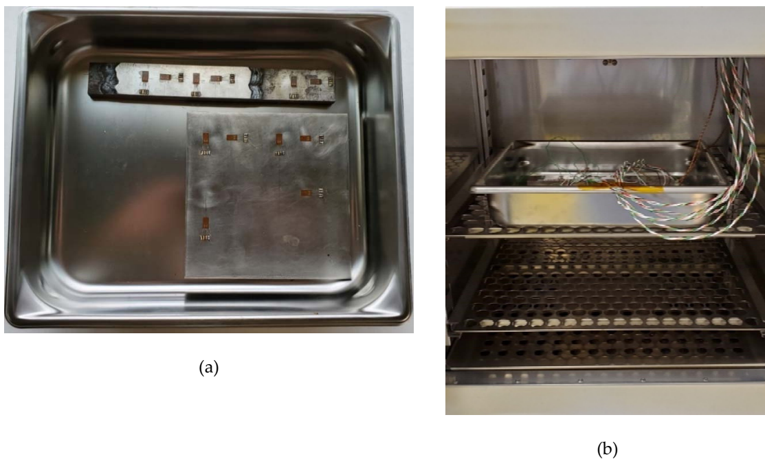
Figure 4. (a) Strain gauges bonded to the machined Invar beads, steel, and Invar reference plate. (b) Invar plates in the oven with strain gauges and thermocouples.
