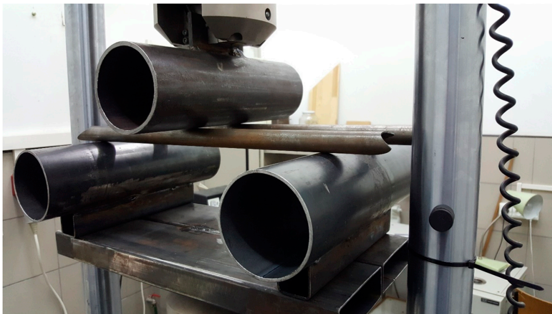
Figure 3. Steel tubes test setup.
