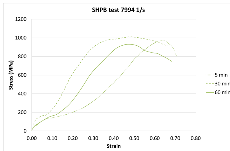
Figure 16. Results of the SHPB test (strain rate of 7994 1/s) of durable resin for curing times of 5, 30, and 60 min for UV and heat exposure.
