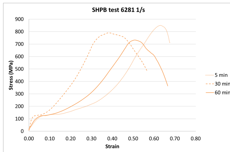
Figure 15. Results of the SHPB test (strain rate of 6281 1/s) of durable resin for curing times of 5, 30, and 60 min for UV and heat exposure.
