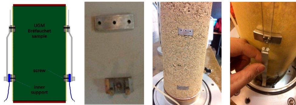
Figure 8. Fixing two vertical displacement transducers with screws.
