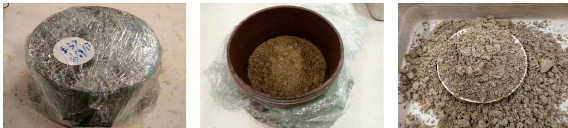
Figure 4. Filter paper method to measure matric suction.
