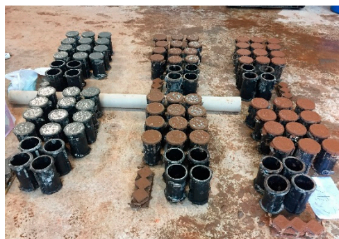
Figure 4. Fabrication of concrete specimens.
