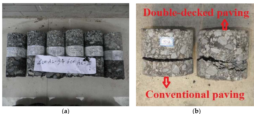
Figure 8. Specimens collected from the trial road constructed by conventional and double-decked paving method: (a) before direct shear test; (b) after direct shear test.
