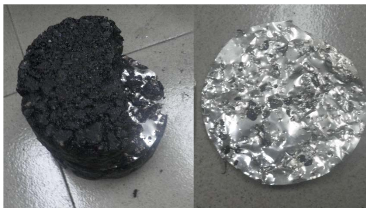
Figure 3. Illustration of the aluminum slice between upper and lower layer of asphalt mixture.
