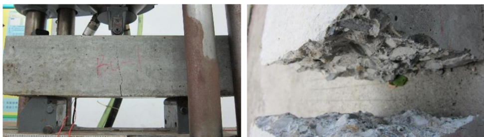
Figure 6. The bending failure mode of the plain concrete.
