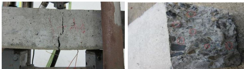
Figure 7. The bending failure mode of BFRC.
