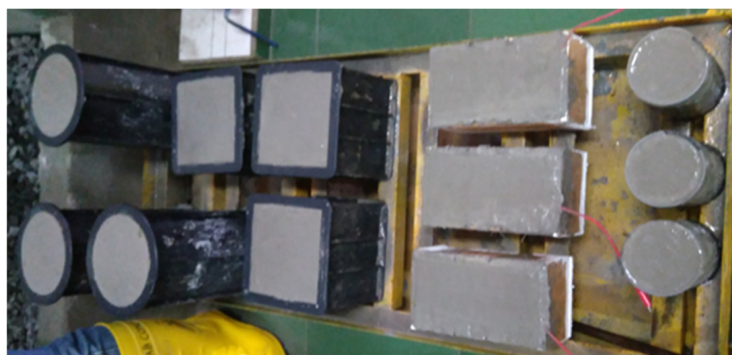
Figure 2. Molds of the specimens after being filled with fresh concrete.
