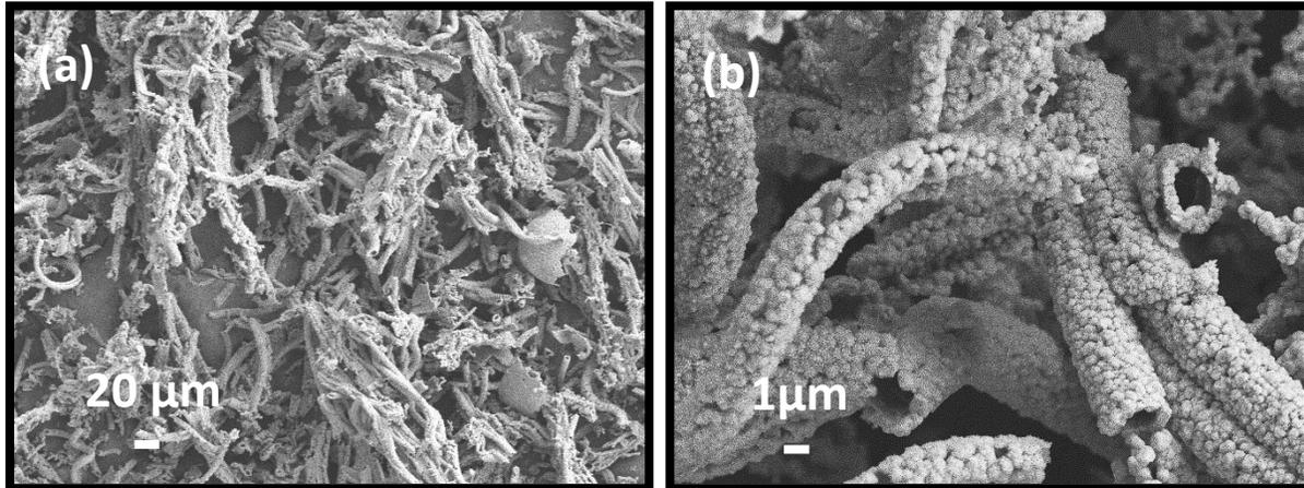
**Figure S3.** FESEM images of calcined fibers obtained with 9.0(w/w) % ITO precursor salts in the spinning solution. Fibers were calcined at 700 °C for 2 h with a heating rate of  $>10\text{ }^{\circ}\text{C min}^{-1}$ . Images at (a) low magnification, and (b) high magnification.
