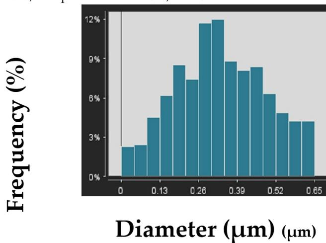
Figure S1. Diameter distribution of ITO nanofibers calcined at 700 °C with a heating rate of 0.5 °C min<sup>-1</sup>.
