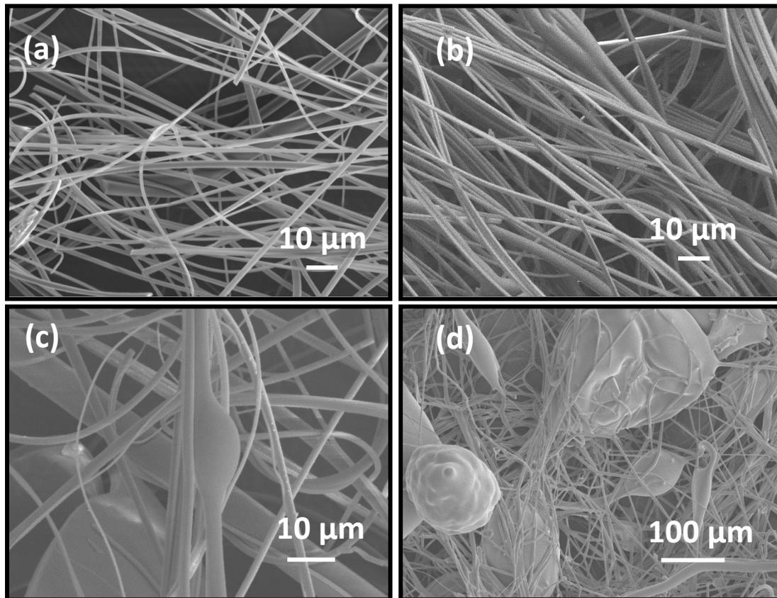
**Figure S2.** FESEM images of polymer precursor fibers obtained from a PVP-InCl<sub>3</sub>-SnCl<sub>4</sub> spinning sol solution containing different (w/w) % of ITO precursor concentration (a) 4.5, (b) 9.0, (c) 12.0, and (d) 18.0. All experiments were performed under identical conditions as mentioned the experimental section.
