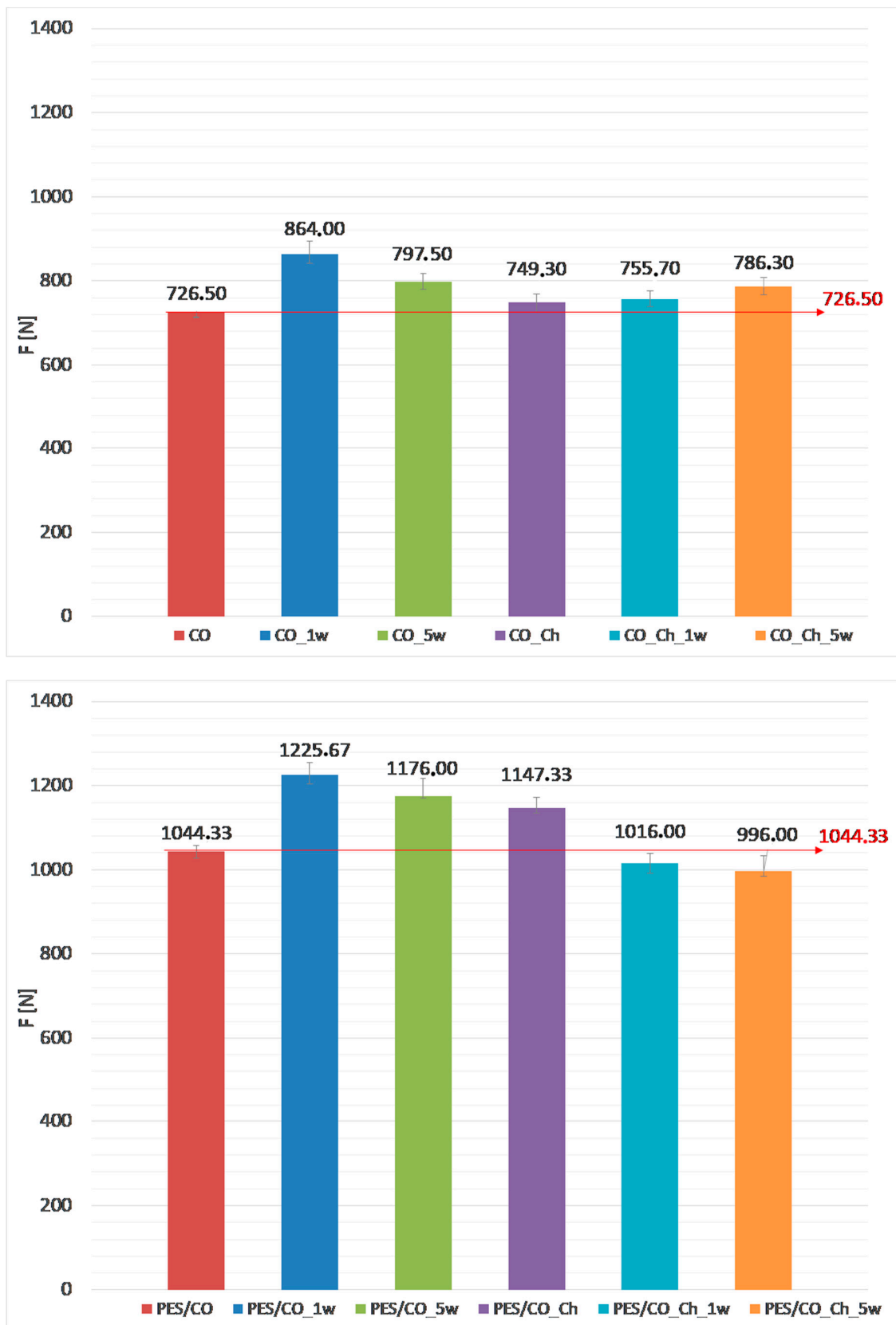
Figure 9. Breaking force, F [N] with interval of confidence (IC99%) of (a) cotton (CO), (b) polyester/cotton blend (PES/CO) fabric before and after washing cycles.
