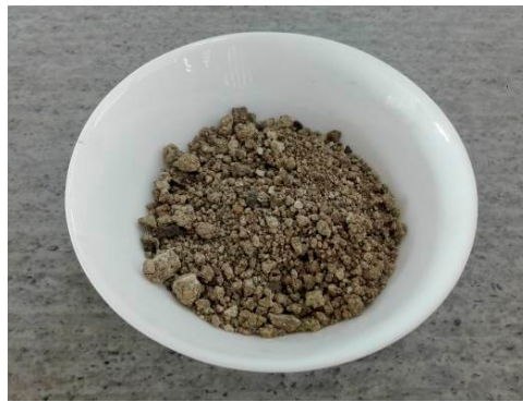
Figure 1. Clay soil 'Cl' from Central Europe (Brno, CZ).
