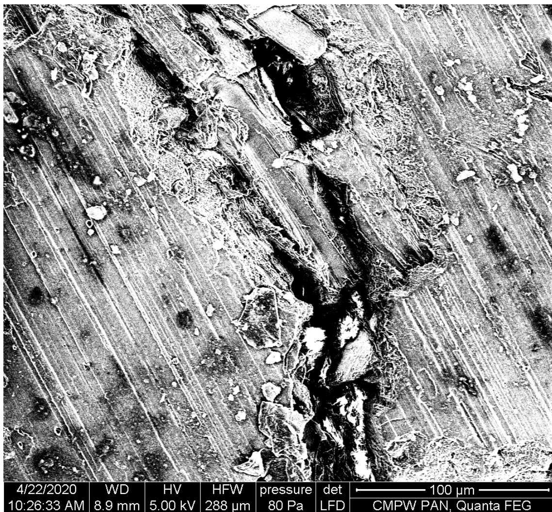
(o) SEM micrographs of the P(3HB-co-4HB)/20WF after 21 days of degradation in water.
