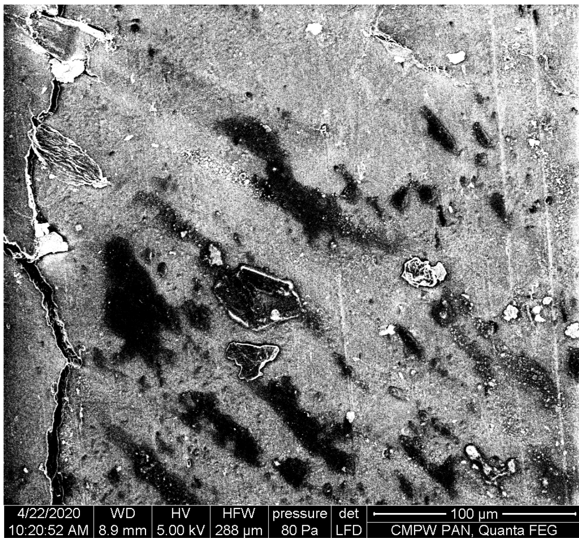
(r) SEM micrographs of the P(3HB-co-4HB)/10WF after 21 days of degradation in buffer.
