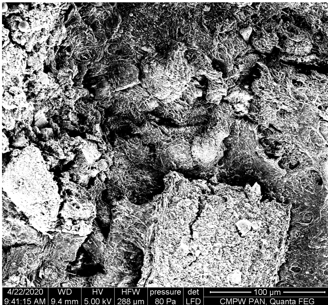
(1) SEM micrographs of the P(3HB-co-4HB)/30WF after 21 days of degradation in Respirometer.
