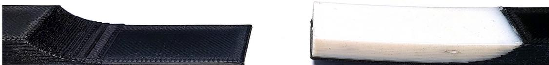
**Figure 1.** Tip of Acoustic Black Holes (ABH) beam with (right) and without (left) additional damping material.
