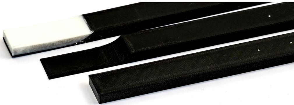
**Figure 2.** Overview of beam specimens with different system complexity: simple beam structure made of PLA (**front**), beam structure with an ABH made of PLA (**center**), and beam structure with an ABH made of PLA with an additional damping treatment made of a thermoplastic polyurethane (**back**).
