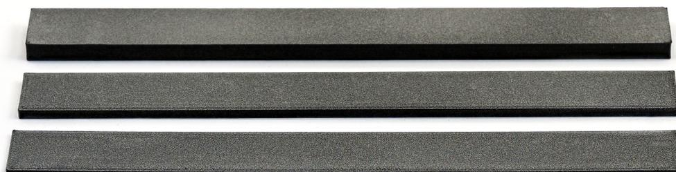
**Figure 3.** Overview of investigated specimen of three different thicknesses (6 mm, 3 mm, 1 mm).
