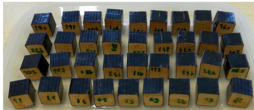
Figure 5. Insulated wood samples.
