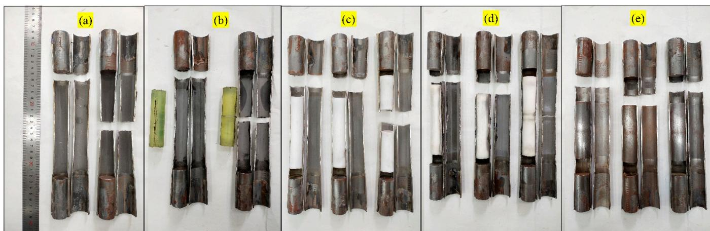
Figure 11. Longitudinal section of the fractured specimen. (a) Longitudinal cross-sectional view of empty tube test specimen. (b–e) The longitudinal cross-sectional views of the specimens when the tube fillers are PU, PTFE, ABS and Q235 respectively.
