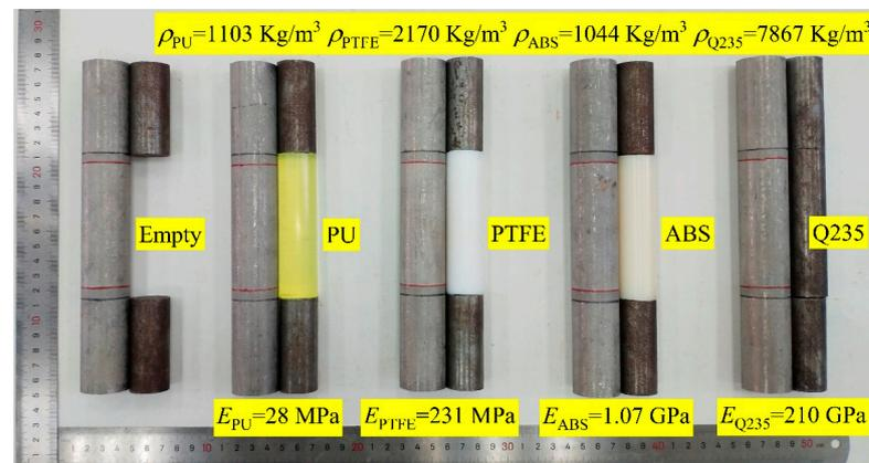
Figure 2. Internal support conditions.
