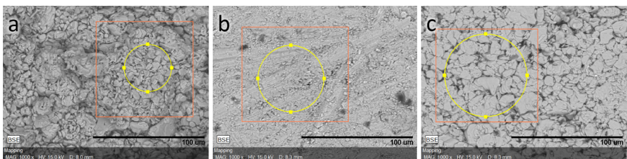
Figure 2. SEM images of \text{CuCrS}_2 samples: powder (a), vacuum compressed (b) and argon atmosphere treated samples (c).
