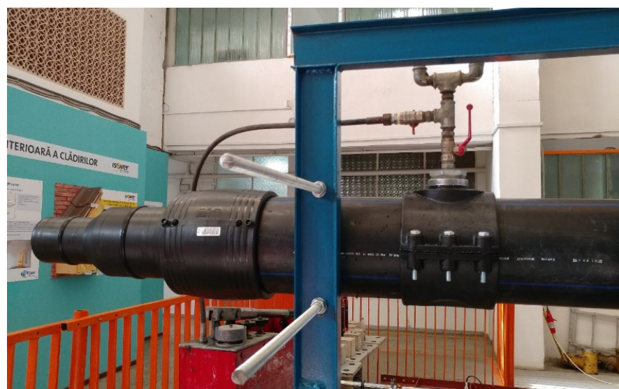
Figure 4. Free end sealing and pressure gauge mounting for internal pressure monitoring.
