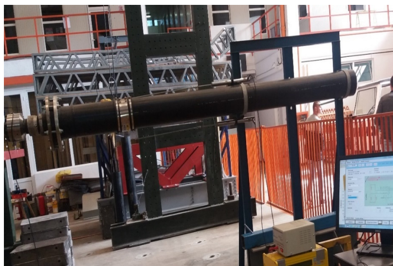
Figure 3. AEP 100 kN Force Cell and Celesco PT5AV Wire Displacement Transducer.
