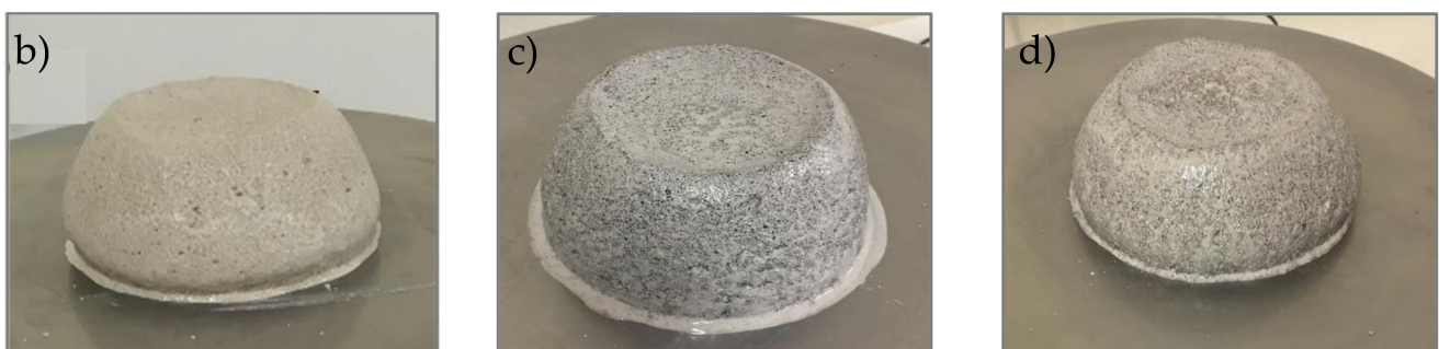
Figure 5. Flow diameters for mortars (a) and final appearance of MW0.29 (b) MCA0.35 (c) and MCT0.33 (d) mortars.
