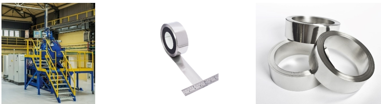
Figure 1. Melt spinning casting setup used in the research, 50.8 mm wide ribbon obtained during the casting, exemplary wound cores prepared for annealing.
