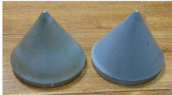
Figure 1. The reactive material liner.
