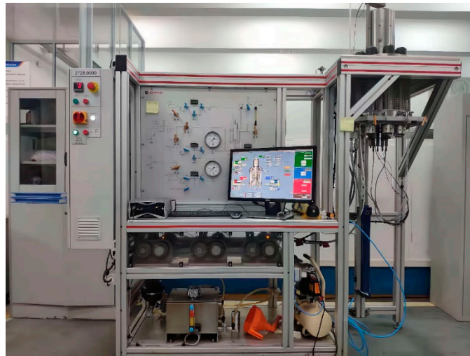
Figure 4. The auto-compensated and auto-equilibrated triaxle cell system.
