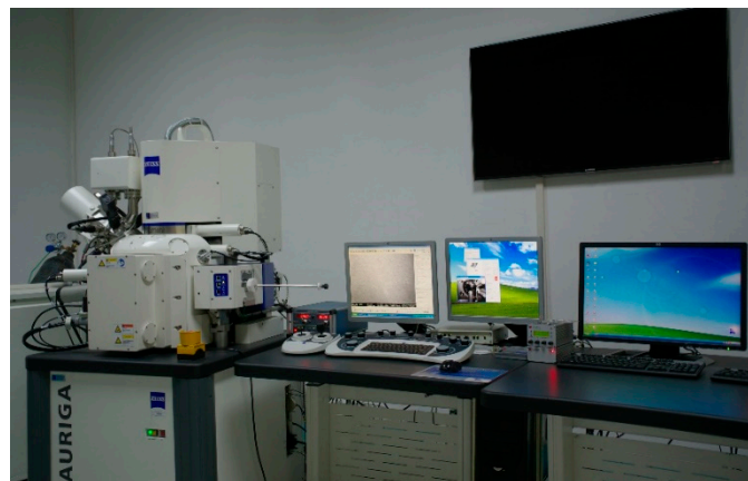
Figure 5. ZEISS Auriga SEM/FIB Crossbeam System.
