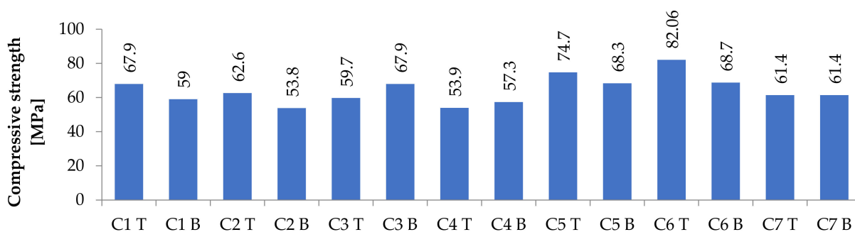
Figure 4. Compressive strength results at the top (T) and bottom (B) parts of columns for individual concrete mixtures.
