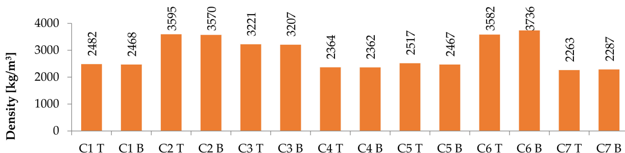
Figure 3. Density results at the top (T) and bottom (B) parts of columns for individual concrete mixtures.
