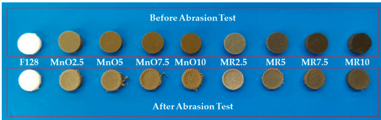
Figure 13. Samples before and after the abrasive wear test.
