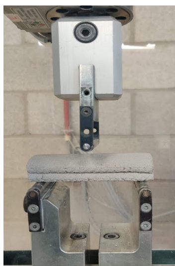
Figure 3. Three-point bending test set-up.
