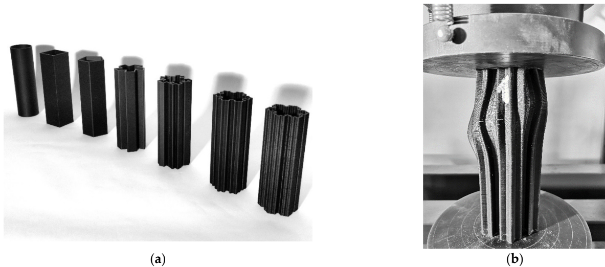
Figure 5. 3D printed column formworks (a); deformation of a concrete-plastic column during compression (b) Images created by A. Skoratko.
