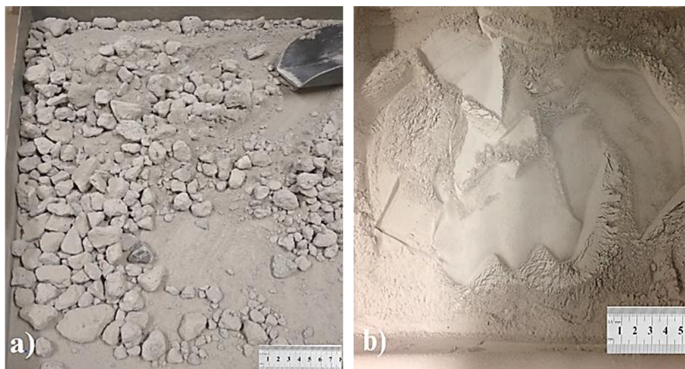
Figure 3. (a) Concrete rubble after thermo-mechanical treatment and (b) recycled fines after grinding.
