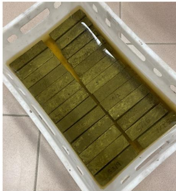
Figure 2. Samples 40 mm × 40 mm × 160 mm during saturation.
