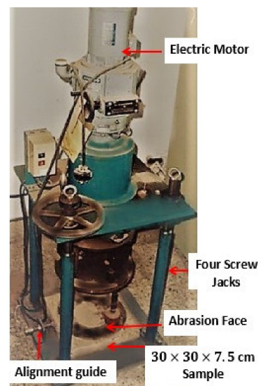
Figure 4. Revolving disk abrasion test machine.
