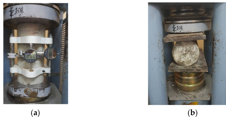
Figure 3. (a) Compression and modulus of elasticity tests, (b) splitting tensile tests.
