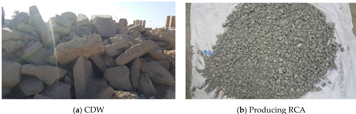
Figure 2. Recycling CDW as concrete aggregate.
