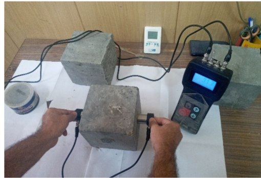
Figure 5. The ultrasound pulse velocity (UPV) tests.
