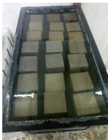
Figure 7. Specimens were immersed in the water tank for the absorption test.
