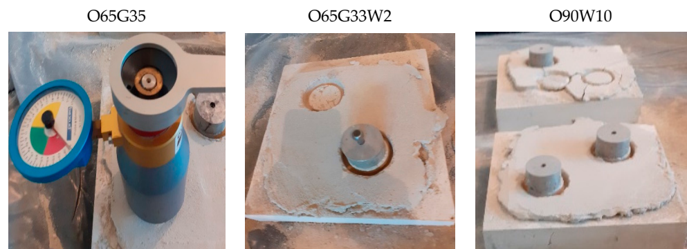
Figure 9. Testing the adhesion of adhesive mortar to concrete.
