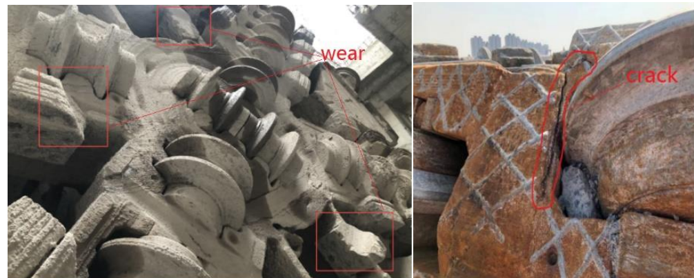
Figure 2. Failed cutterhead of a shield machine.
