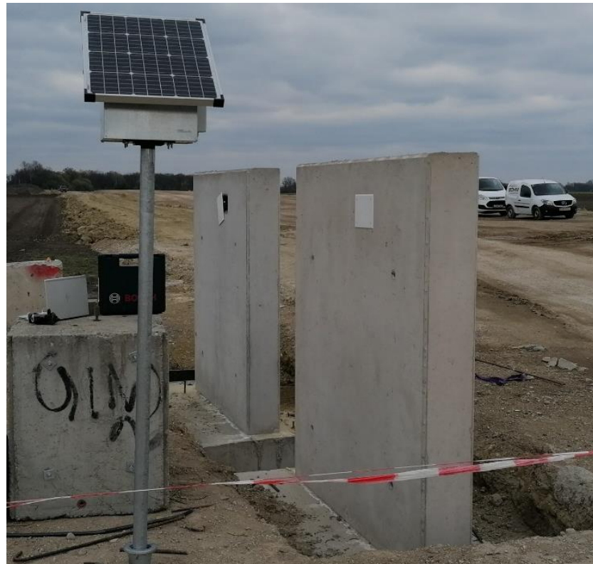
Figure 12. Mock-up walls in standard concrete and Eco-concrete for monitoring and long-term tests (© Autischer, IMBT).
