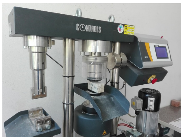
Figure 7. Mortar strength tests—a compression mortar test stand.
