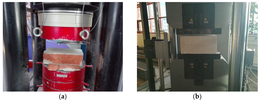
Figure 13. Strength tests of masonry units: (a) tests of solid bricks, (b) tests of autoclaved aerated concrete blocks.
