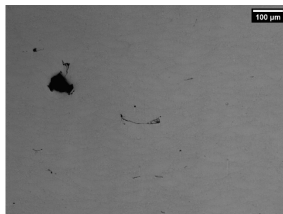
Figure 11. Cross-section morphology of sample built with P = 85\text{ W} , v = 650\text{ mm/s} and hd = 70\text{ }\mu\text{m} .
