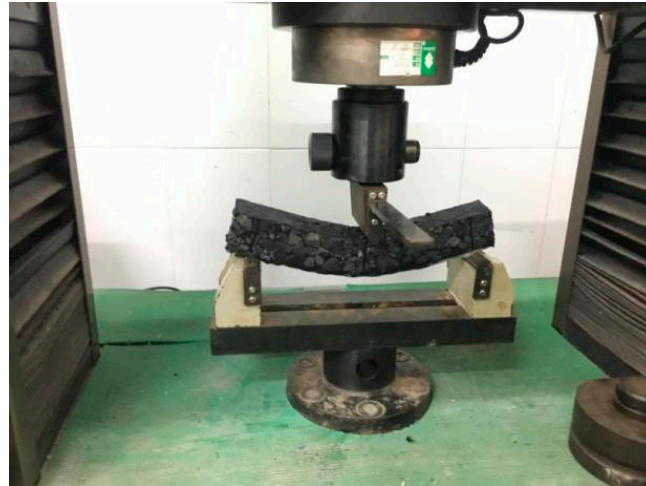
Figure 6. Three-point bending test.
