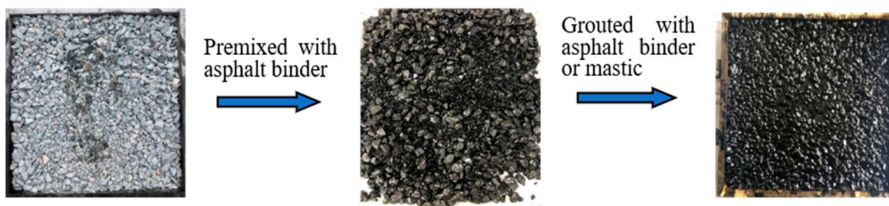
Figure 2. Flow chart of the grouting scheme.
