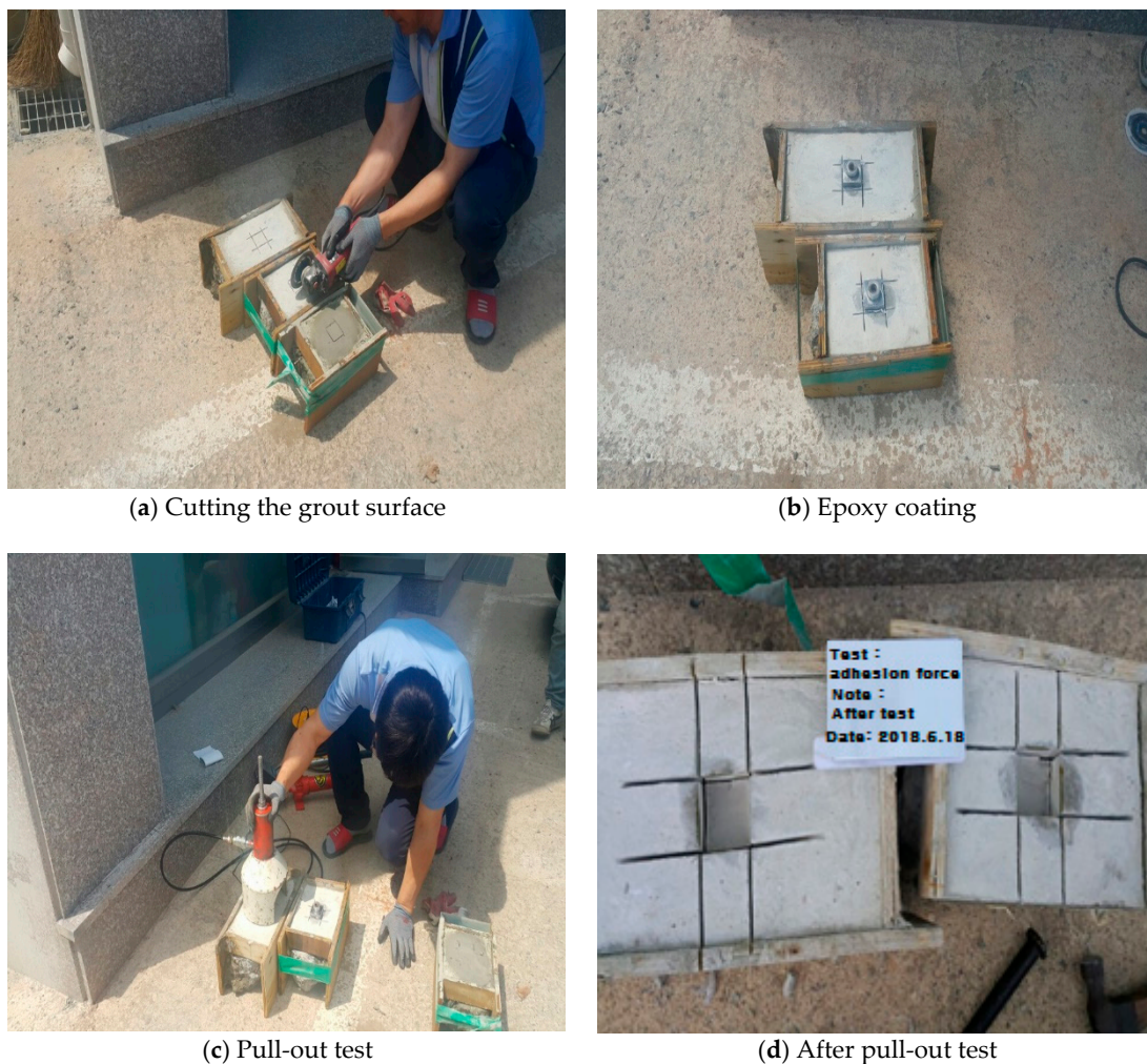
Figure 6. A view of the test to check the adhesion force.
