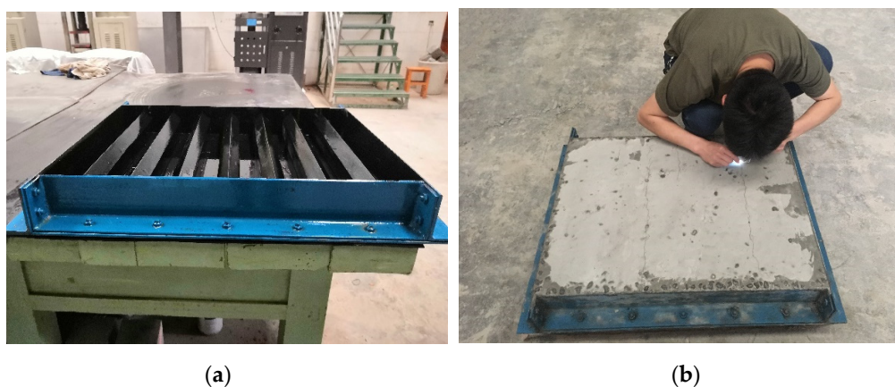
Figure 10. Cracking sensitivity experiment: (a) blade mold; (b) crack observation.
