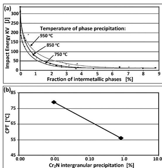
**Figure 8.** Changes in the microstructure lowering ductility and corrosion resistance of duplex steels, including (a) breaking energy KV as a function of intermetallic phase content in duplex steels (according to [37]), (b) CPT (Critical Pitting Temperature) index as a function of the content of intercrystalline  $\text{Cr}_2\text{N}$  precipitates (according to [38]).
