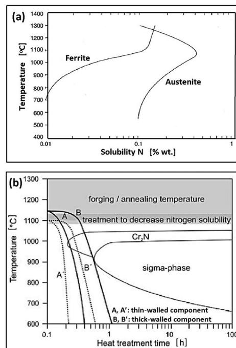
**Figure 10.** Heat treatment of duplex steel, including (a) solubility of Nitrogen in ferrite and austenite (according to [38]), (b) heat treatment of the thin-walled and thick-walled duplex steel elements (according to [23]).
