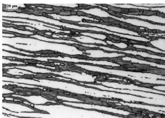
**Figure 2.** A properly balanced duplex steel microstructure containing approximately 50% of each  $\delta$ -ferrite (dark areas) and  $\gamma$ -austenite (light areas)—according to [21].
