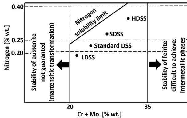
Figure 3. Stability areas of conventional duplex steels—according to [21].
