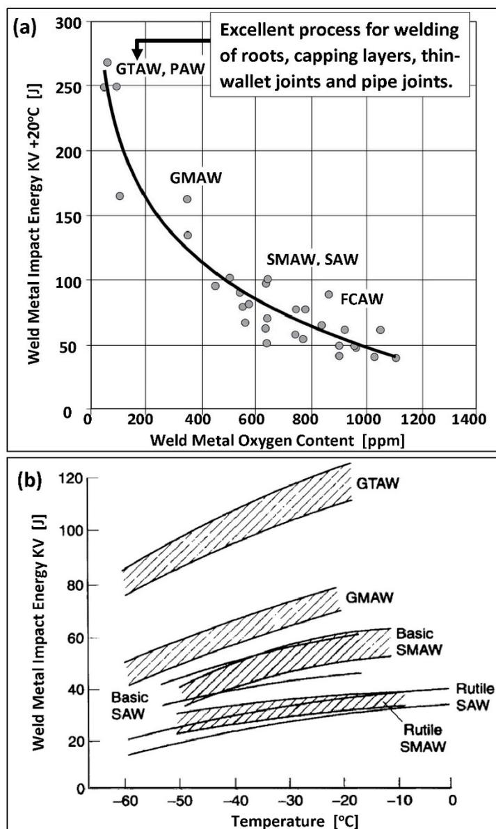
**Figure 14.** Breaking energy of the weld metal: (a) breaking energy KV determined at 20 °C as a function of oxygen content in the duplex weld metal, (b) breaking energy KV determined at 0–(–60) °C, specified for various welding methods (according to [28]). The meaning of individual abbreviations is explained in the Abbreviations of this paper.
