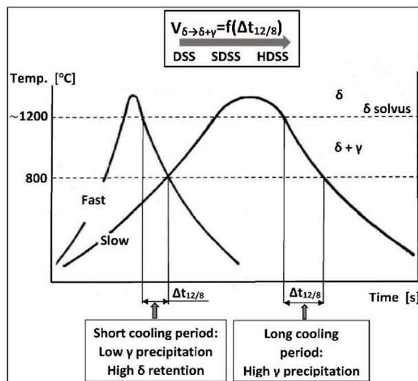
**Figure 6.** Influence of cooling rate on the content of  $\delta$ -ferrite in duplex steels (according to [30]). Left-hand frame: fast cooling, high  $\delta$ -ferrite content; right-hand frame: slow cooling, high content of  $\gamma$ -austenite precipitates.
