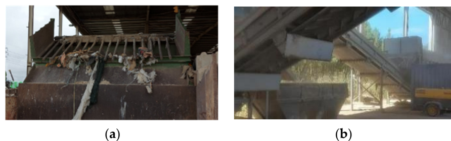
Figure 2. Initial sieving at the feeder (a) Removal of large and elongated materials with bar sieve (b) Removal of finer materials.
