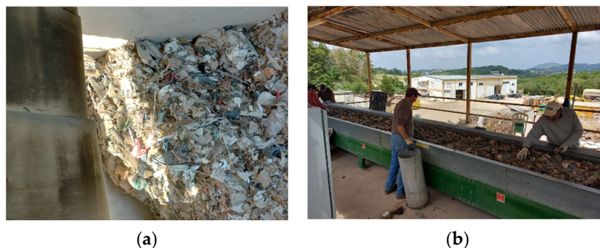
Figure 4. Traditional processes for the removal of unintended constituents (a) Lightweight materials removed by air sifting (b) Hand sorting.
