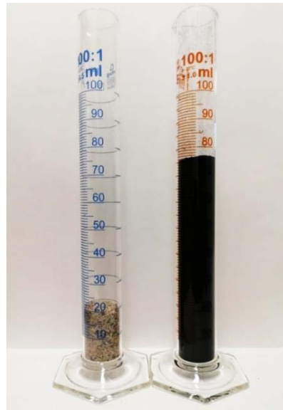
Figure 5. Volume difference between sand (left) and crumb rubber (right) of the same weight (10 wt %).
