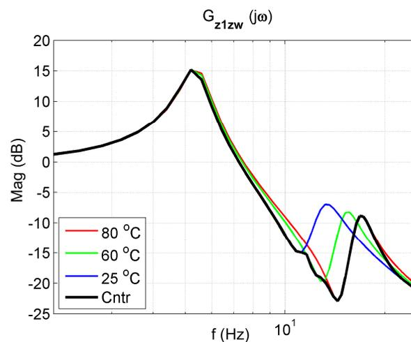
**Figure 19.** Vibration transmissibility functions of disturbance  $z_w$  to the protected mass  $m_1$  of the passive absorber for selected temperatures of 25 °C, 60 °C, 80 °C and the controlled absorber (black). The transfer function  $G_{z1zw}$  describes the object.
