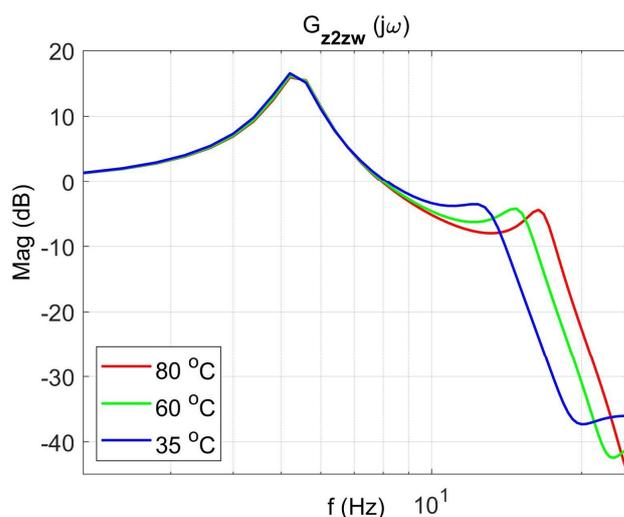
Figure 14. Vibration transmissibility functions of disturbance  $z_w$  to the absorber mass  $m_2$  as a function of frequency for selected temperatures 25 °C, 60 °C, 80 °C, the transfer function  $G_{z2zw}$ .
