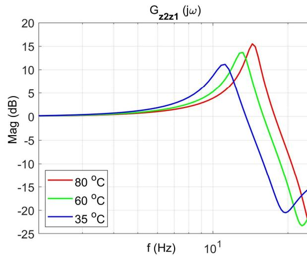
Figure 6. Vibration transmissibility functions of the absorber as a function of frequency for selected temperatures 25 °C, 60 °C, 80 °C, the transfer function  $G_{z2z1}$ .
