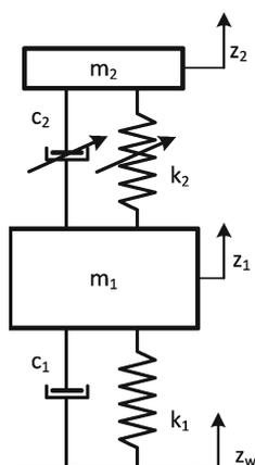
Figure 3. Calculation diagram of the vibration reduction system.
