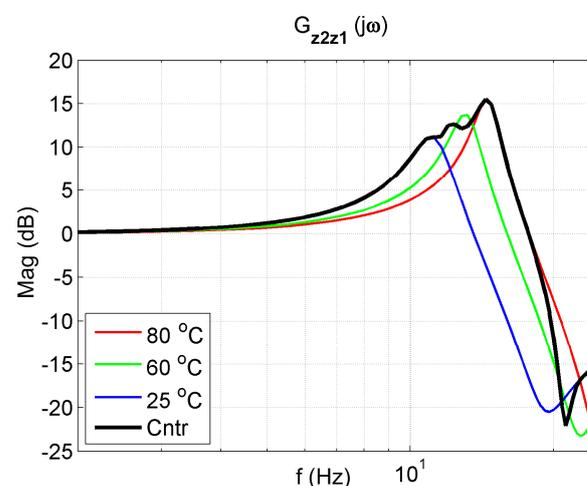
**Figure 18.** Vibration transmissibility functions of the passive absorber for selected temperatures of 25 °C, 60 °C, 80 °C and the controlled absorber (black). The transfer function  $G_{z_2 z_1}$  describes the object.
