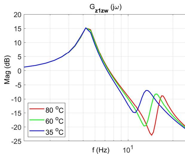
Figure 10. Vibration transmissibility functions of disturbance  $z_w$  to the protected mass  $m_1$  as a function of frequency for selected temperatures 25 °C, 60 °C, 80 °C, the transfer function  $G_{z1zw}$ .
