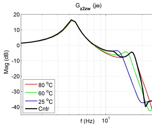
**Figure 20.** Vibration transmissibility functions of disturbance  $z_w$  to the mass  $m_2$  of the passive absorber for selected temperatures of 25 °C, 60 °C, 80 °C and the controlled absorber (black). The transfer function  $G_{z2zw}$  describes the object.
